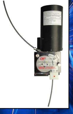
The WF-200<sup>™</sup> drive produces a positive, slip free drive force to the filler material, without damaging or flattening the wire surface. This provides exceptional feeding capability of "soft" wires such as aluminum and copper. The Capstan drive wheel plastically deforms the wire which removes residual cast and permits precise wire placement in the weld puddle.
